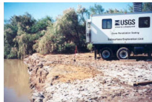
Fig. 8: Steep bank of Alamo River with USGS CPT rig conducting a sounding at WLA site
